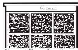
Clogged filter—Greatly reduces cooling, heating and airflow.
