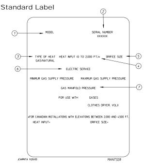
When contacting Maytag, the information on the data label is required to ensure proper service/parts assistance. The data label is located at the lower left rear of the dryer behind the back guard.
