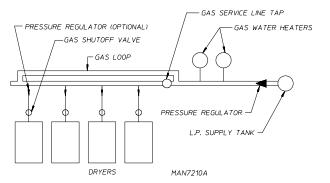
Consistent gas pressure is essential at all gas connections. It is recommended that a 3/4-inch (19.05 mm) pipe gas loop be installed in the supply line servicing a bank of dryers. An in-line pressure regulator must be installed in the gas supply line (header) if the (natural) gas pressure exceeds 13.0 in wc (32.34 mb) pressure.
