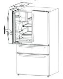
5. Remove the 4 hex head bolts hinges (I) with an Allen wrench (5 mm).Remove the lower left and right door hinges (J).
