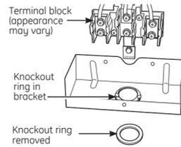
**C** For power cord installations only (see the next step if using conduit), assemble the strain relief in the hole. Insert the power cord through the strain relief and tighten. Allow enough slack to easily attach the cord terminals to the terminal block. If tabs are present at the end of the winged strain relief, they can be removed for better fit.
