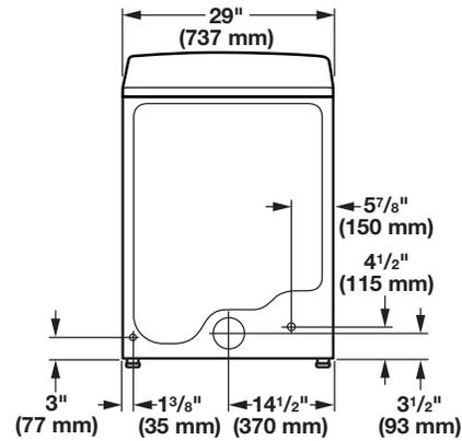
**NOTE:** Leveling legs 1" (25 mm) (3.6 washer capacity) or 1<sup>1</sup>/<sub>2</sub>" (38 mm) (3.8 washer capacity) depending on model.
