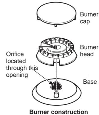
B. Using a 7 mm or 9/32" nut driver, remove the top burner orifices. These may be accessed through the burner opening in the base.
