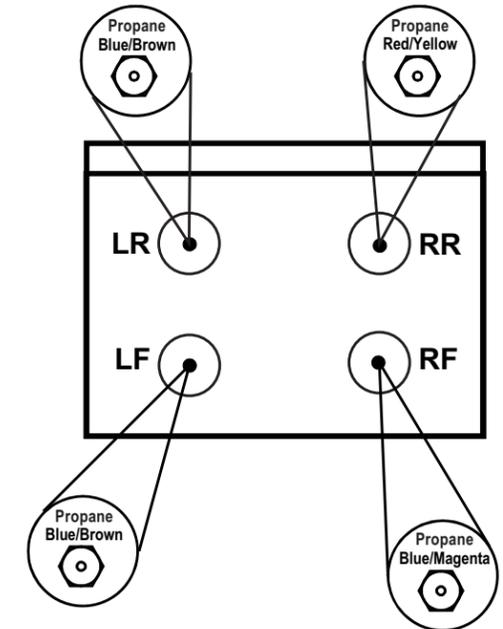
To prevent leakage, make sure the orifice spuds are securely screwed into the gas supply tubes.
